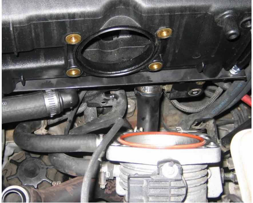
If you buy the m50manifold.com kit a properly designed throttle body seal is included as part of the kit contents. Photo right. It is nearly double the size of the OE seal but not quite. Believe it or not some people even forget to use the m50manifold.com seal even though it comes with their kit.
